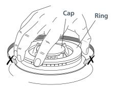
Fig. 21 Correct positioning of cap and ring - triplering wok burner
